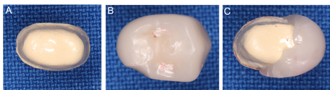
Figure 3. The different fracture patterns of samples. (A) Adhesive. (B) Cohesive, (C) Mixed failures.
