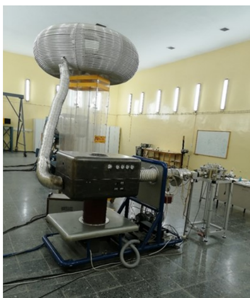
Figure 1. Low Energy Ion Accelerator- Sames J-15 and Van-de Graaff Generator
